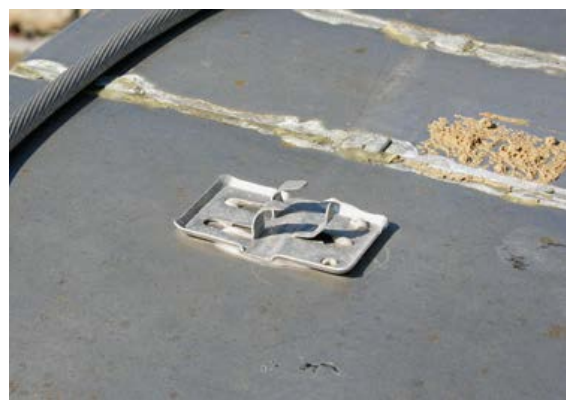
Conductor separated from clip after high wind
