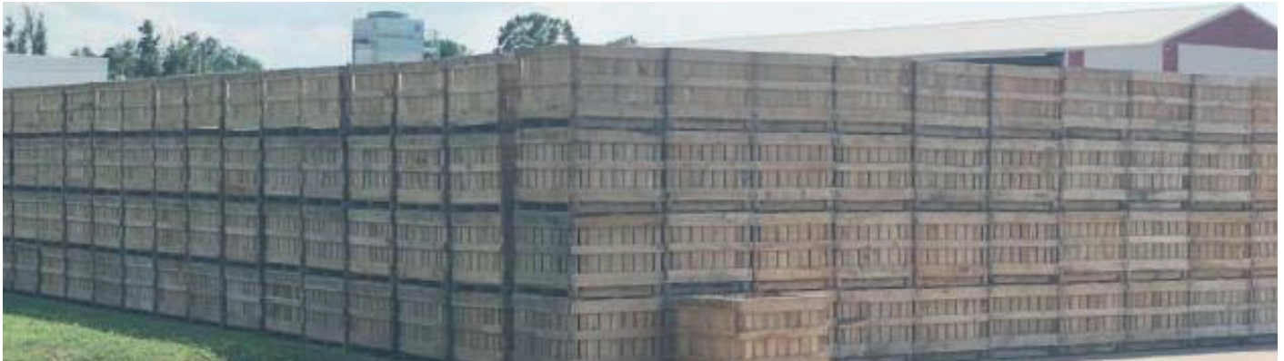
Combustible yard storage, wood bins (Photo source: Rich Gallagher, The Zurich Services Corporation)
